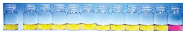
Fig. 1 Color changes of a 10^{-4} M solution of 3 in EtOH– \text{H}_2\text{O} 1 : 1 in the presence of 1 equiv. of every cation as perchlorate or triflate salts.
